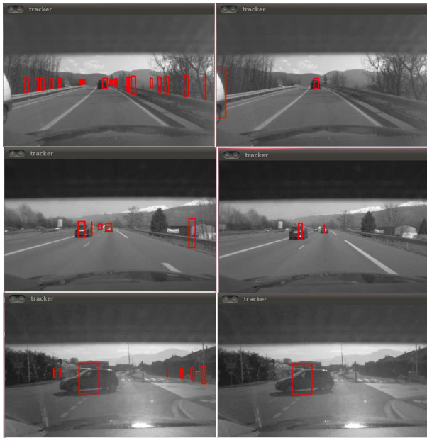
Fig. 9. Example tracking results. For each scenario : Left, FCTA results without motion detection module activated; right, same scenario with motion detection module activated.
