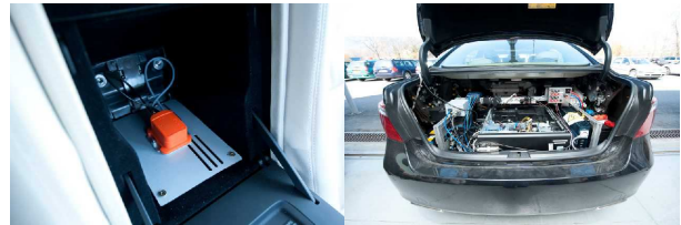
Fig. 6. (left) the MTi-G Xsens IMU unit, (right) the trunk of the car, including the PC used for calculation.
