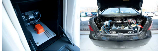
Fig. 6. (left) the MTi-G XSens IMU unit, (right) the trunk of the car, including the PC used for calculation.
