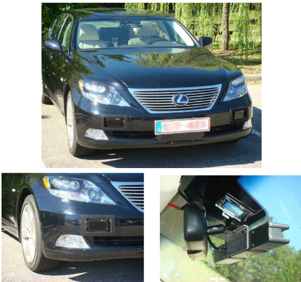
Fig. 5. Lexus LS600h car equipped with two IBEO Lux lidars and a TYZX stereo camera
