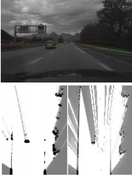
Fig. 1. (up) Left image from the stereo camera. (down) Occupancy grids computed from multiple layers of laser scans: (left) with Bayesian Fusion, (right) with our new approach. Due to conflicting information, the left fence disappears with Bayesian fusion, while still being visible with our method.
