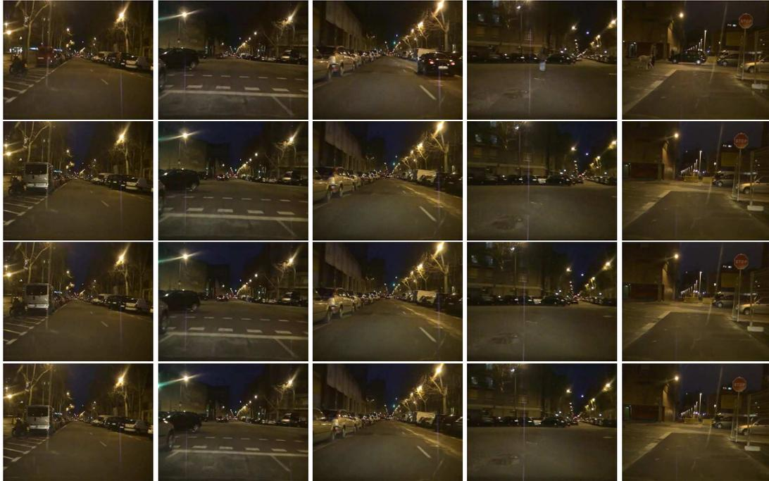
Figure 3: (First row) Query (current) frames of *Night1* sequence and synchronization results obtained by (second row) exhaustive search, (third row) SIFT-based retrieval and (fourth row) SURF-based retrieval.
