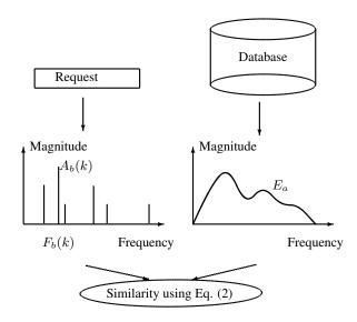
**Fig. 1.** Schema of the proposed approach. The request is represented as an irregularly sampled spectral envelope (stems) whereas the records of the database are represented as a regularly sampled one (solid line).
