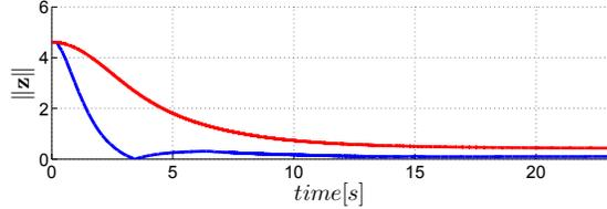
Fig. 3: Behavior of the estimation error  $z(t) = \chi(t) - \hat{\chi}(t)$  when actively optimizing the camera motion for improving the estimation convergence rate (case 1 – blue line) and when not optimizing the camera motion (case 2 – red line).
