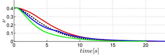
Fig. 2: Behavior of the error norm  $\nu(t)$  when using: the full strategy of Secs. III-B and III-C and the estimated  $\hat{\chi}(t)$  (case 1 – blue line); the classical controller (9) and the estimated  $\hat{\chi}(t)$  (case 2 – red line); the classical controller (9) by employing  $\hat{\chi} = \chi^*$  (case 3 – green line); the classical controller (9) by using the real  $\chi(t)$  (case 0 – black dashed line)
