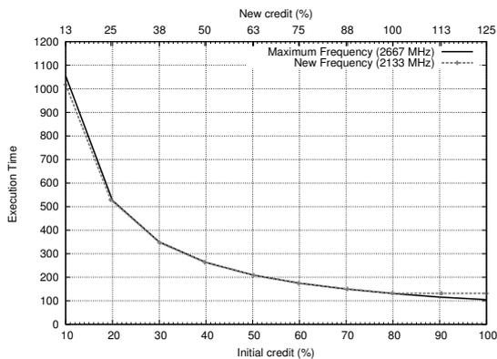
Fig. 1. Compensation of Frequency Reduction with Credit Allocation
