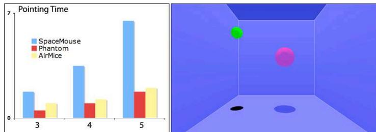
**Fig. 5 Left:** Mean Pointing Time (in seconds) for each device and for each ID. Subjects are slower with the SpaceMouse and faster with the PHANTOM. AirMouse is placed in between, but closer to the PHANTOM. **Right:** Snapshot of the 3D pointing evaluation environment. The green sphere on the left must be moved as fast as possible into the transparent red area. The transparent area size is modified during the experiment for defining different difficulties (IDs).
