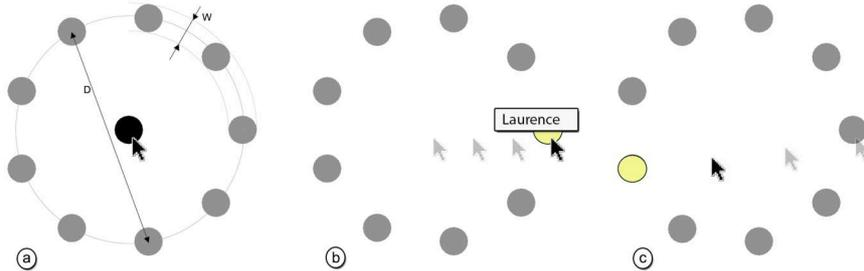
**Fig. 3** Combination of multidirectional tapping with click-and-write. **a:** Initial cursor position, with amplitude and width visual representation. **b:** First target is reached (and clicked), the subject wrote her first name. **c:** 'RETURN' has been pressed, the cursor is going to the next target.
