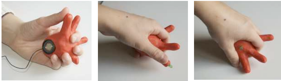
Fig. 10. Design alternatives for output ports: sound (left), light (LEDs in center and right). Focusing on the output ports: according to the way the tool is handled by the user, the lights may be hidden or not.
