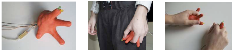
Fig. 9. Roam tool prototypes: close-up of final prototype with bend sensors and green/yellow LEDs (left), in the hand of the user (center). Another prototype of the Roam tool with separated physical properties (right).
