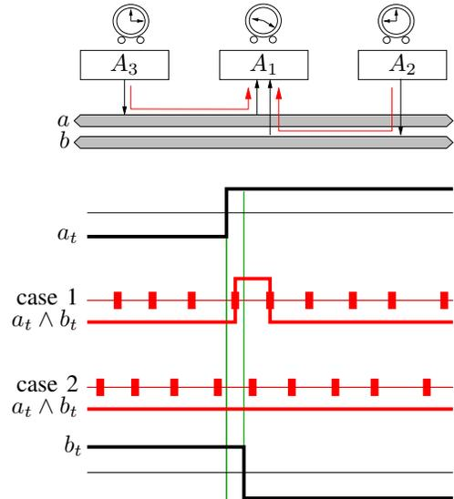
Figure 2. Sensing multiple signals, for distributed clocks subject to independent drifts and jitters. Referring to Figure 1, we show the case of  $A_1$  reading two boolean inputs originating from  $A_2$  and  $A_3$ , respectively, and computing their conjunction. Cases 1 and 2 correspond to two different outcomes for the local clock of  $A_1$ .
