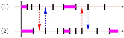
Figure 8. Synchronization principle used in time-based LTTA.
