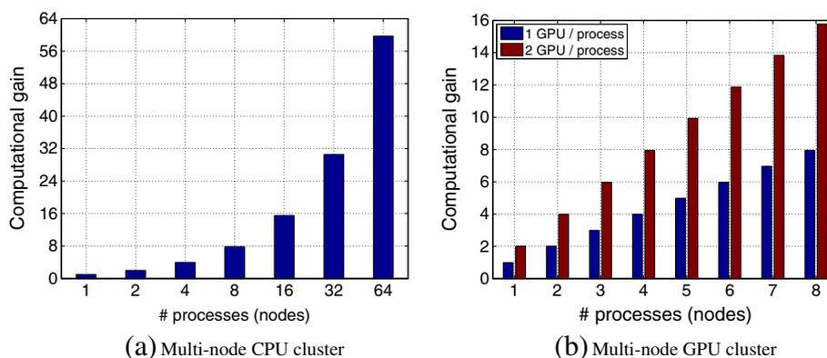
**Figure 4** The speed-up obtained when using (a) a 64-node CPU cluster and (b) an 8-node GPU cluster to calculate 14,630 2D single-precision NCCs of size 4096 × 4096. Here, the number of threads in each process is equal to the number of CPU cores per node in (a), and the number of GPUs per node in (b).
