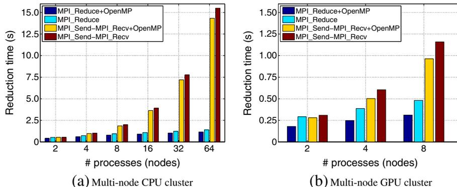
**Figure 5** The reduction time on (a) Griffon (64-node cluster, 20Gb/s InfiniBand), and (b) Adonis (8-node GPU cluster, 40Gb/s InfiniBand) using different inter-process communication strategies (i.e. the MPI\_Reduce or MPI\_Send and MPI\_Recv functions), and different methods for calculating the reduce operation on each node (i.e. with or without using OpenMP parallelisation). Note that the time axis in (b) is 10× smaller than in (a).
