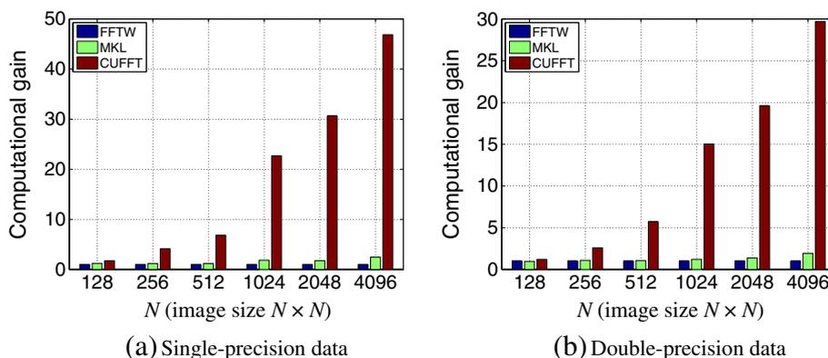
**Figure 2** Comparison of the relative speed of 2D FFT NCC single-precision (a) and double-precision (b) calculations at different micrograph sizes  $N \times N$  (pixels) using the MKL, FFTW libraries on one CPU core of our Dirac workstation (3.2GHz i7-965) and the CUFFT library on one C2075 GPU (448 cores). The size of template images are chosen as  $N/8 \times N/8$ . All timings are normalised to the FFTW (one unit).
