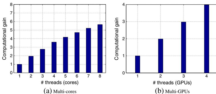
**Figure 3** The speed-up obtained by using multi-threading to calculate 14,630 2D single-precision NCCs of size  $4096 \times 4096$  on (a) a dual quad-core workstation (Dirac), and (b) a four-GPU server (Mbiserv). See Table 1 for hardware details.
