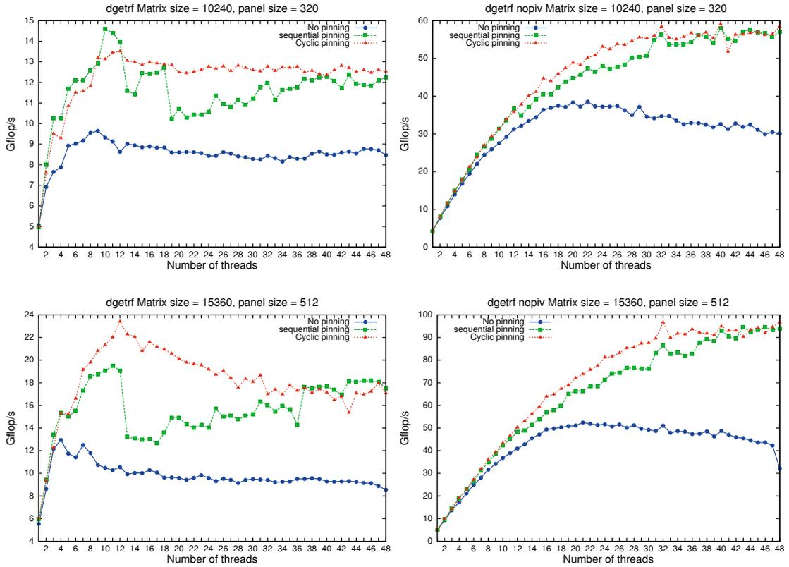
Figure 3: Performance of thread pinning strategies for LU panel factorization with pivoting (left) and no pivoting (right). Panel sizes:  $10240 \times 320$  and  $15360 \times 512$ .
