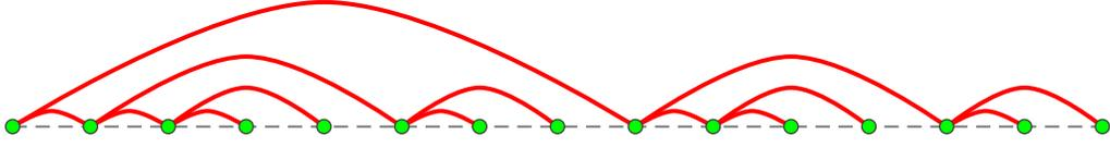
Fig. 5: 1-stack layout of a complete binary tree.
