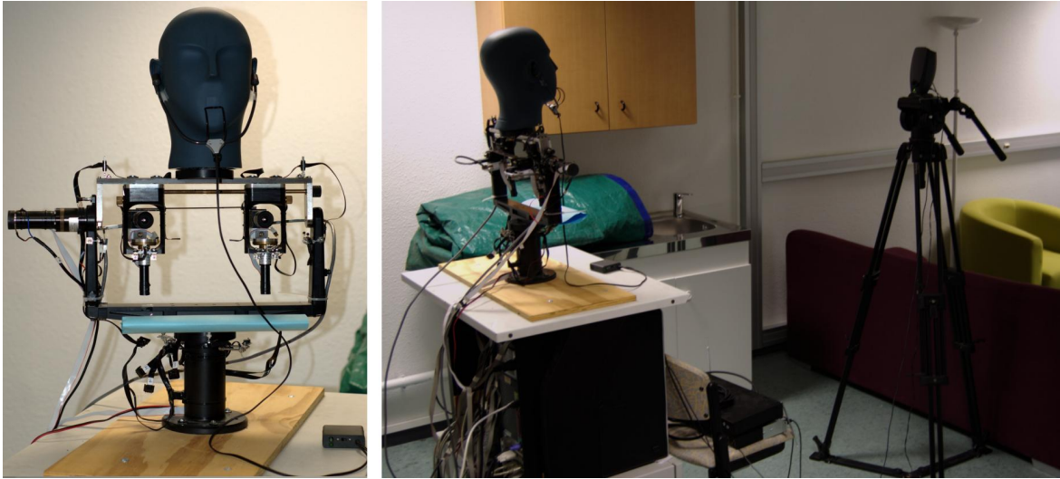
Fig. 1: A binaural dummy head is placed onto a motor system which can perform precise and reproducible pan and tilt motions (left). The emitter (a loud-speaker) is placed in front of the robot (right).
