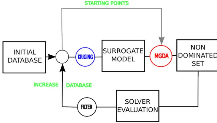
Figure 4: Global procedure for kriging-assisted *MGDA* optimization.
