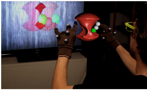
Figure 2: Illustration of a virtual design immersive system based on natural bimanual interactions proposed in [32]
