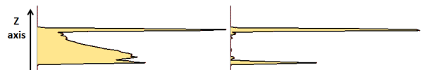
Figure 2: Cluttered and uncluttered distributions. Comparing point distributions along vertical direction n_z without filtering by normals (left) and with filtering by normals (right, |n_i \cdot n_z| > 0.98 ). The chosen bin size is 8 cm and the distribution is split into 69 bins.
