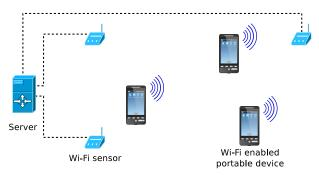
Figure 1: Architecture of a Wi-Fi tracking system.
