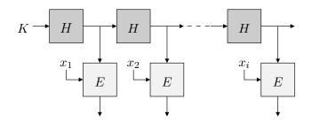
Figure 6: Anonymization using a hash chain and a block-cipher for a sequence of addresses  $(x_1, x_2 \cdots x_i)$ .
