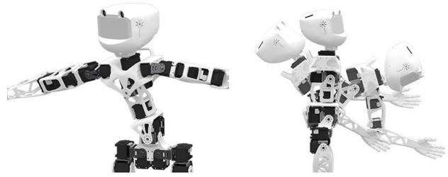
Fig. 2: These figures illustrate some morphological features of the Poppy humanoid Robot: Poppy has an articulated trunk of 5 DoFs which allows more natural and fluid motions while improving the user experience during physical interaction and actively participating to the balance of the robot.
