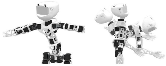
Fig. 2: These figures illustrate some morphological features of the Poppy humanoid Robot: Poppy has an articulated trunk of 5 DoFs which allows more natural and fluid motions while improving the user experience during physical interaction and actively participating to the balance of the robot.
