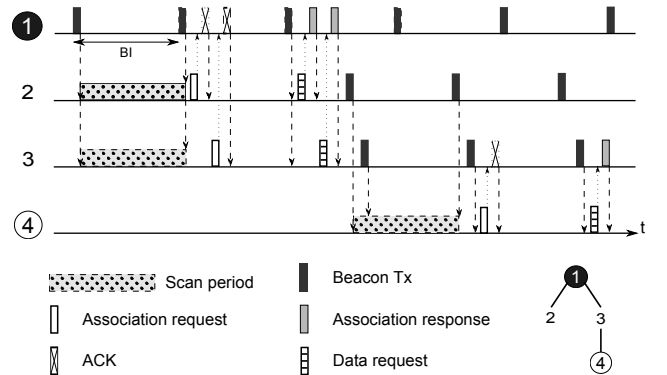
Fig. 1: Topology construction in an example 802.15.4 cluster-tree.
