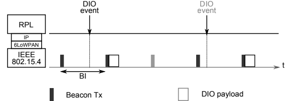
Fig. 2: Encapsulation of DIO messages in beacon frames.
