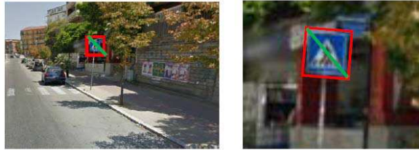
Fig. 6: Target reachability. On the left side, the target is supposed unreached since the green diagonal length is under a threshold. On the right side, the target is considered to be close enough and reached.
