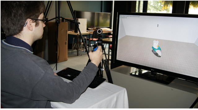
Figure 6: Experimental setup. Users are seated in front of a screen displaying the simulation. They can rest their arm on a table. A keyboard with marked keys allows them to enter their answers.
