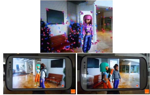
Fig. 7. System in action an indoor scene (top image shows the keypoints used in the relocalisation process).
