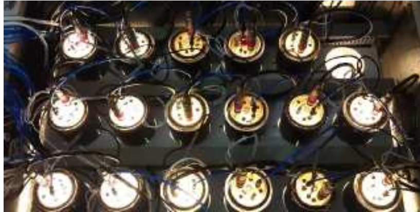
Figure 1: The TIP system. The device has 18 batch photobioreactors for microalgae cultivation.
