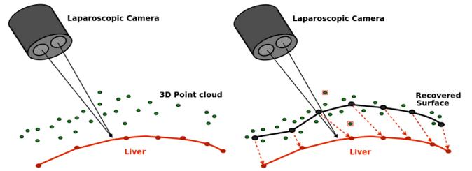
Fig. 2. MLS-based surface recovery. **Left:** Three-dimensional sparse point cloud recovery. **Right:** outliers filtering and surface reconstruction using MLS, the control points selected after clustering are registered to the biomechanical model of the liver
