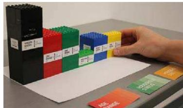
**Figure 4:** placing blocks on sensor pad to answer query (which radio station had the greatest number of male listeners between the ages of 44 to 55.)
