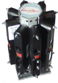
Fig. 5. Omnidirectional RGB-D camera rig.
