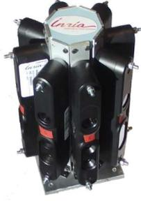
Fig. 5. Omnidirectional RGB-D camera rig.
