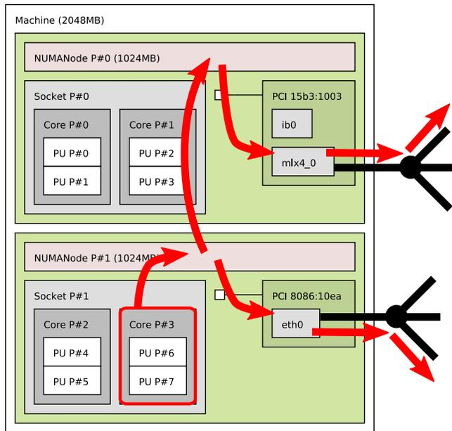
Figure 3. Paths from an hwloc core to a remote object. The Ethernet path goes directly from the local NUMA node to the `eth0` device, and then out to the wire. The InfiniBand path has to cross a NUMA link before it reaches the `mlx4_0` device, and then out to the wire.
