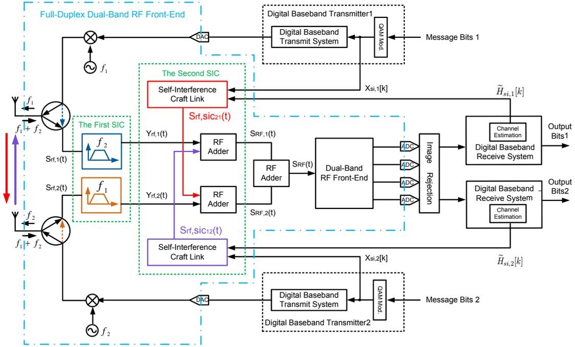
Figure 3: Full-Duplex Dual-Band radio transceiver
