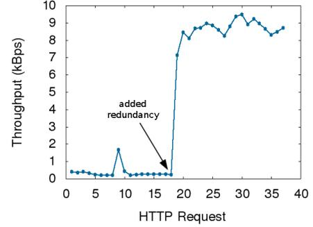
Fig. 7. Throughput before and after the event of activating a redundant gateway with no QoS enforcement policy.
