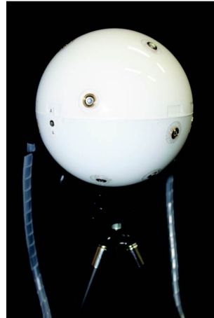
Fig. 1 Fabricated 12-element spherical microphone array of diameter 15 cm. The microphones are mounted on a rigid spherical shell.
