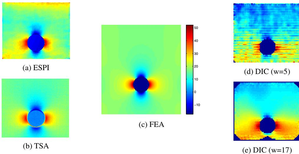
Figure 2: Various measurements and an FEA prediction of the bulk-stress field in a uniaxially loaded plate containing a hole (scale is in MPa).
