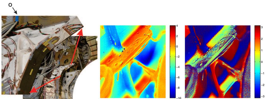
Figure 3: Aircraft related case studies in TSA applied using microbolometers. Scans show thermoelastic response and phase in the case of (a) and (e). The scales are respectively temperature in arbitrary units and radians.
