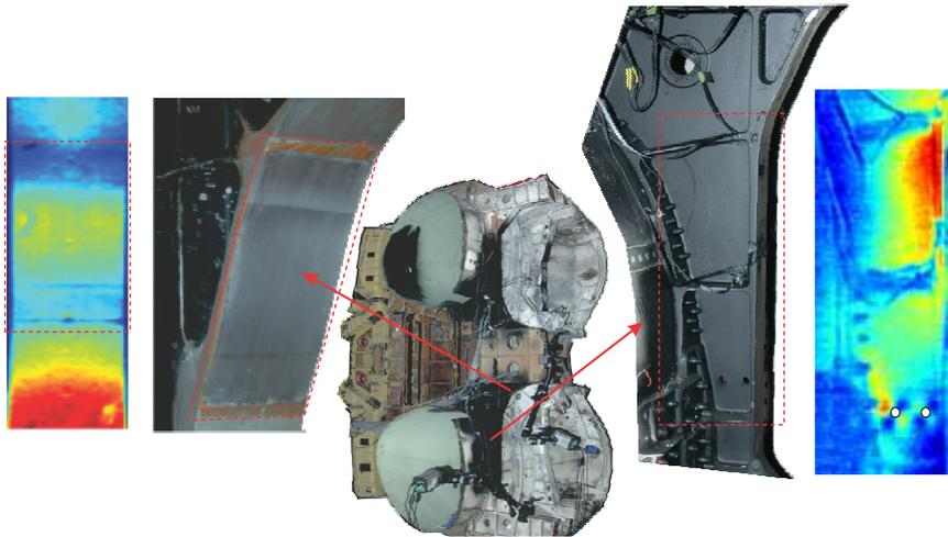
Figure 4: F/A-18 centre barrel on its side with a pair of FLIR A20 microbolometers mounted to the rear bulkhead. The two areas of interest are the main landing gear pocket area (right photo) and an adhesively bonded metallic patch to the kick point flange (left photo). The scans show the thermoelastic response under a  $\approx 1$  Hz sinusoidal load at 8% of the peak spectrum load.
