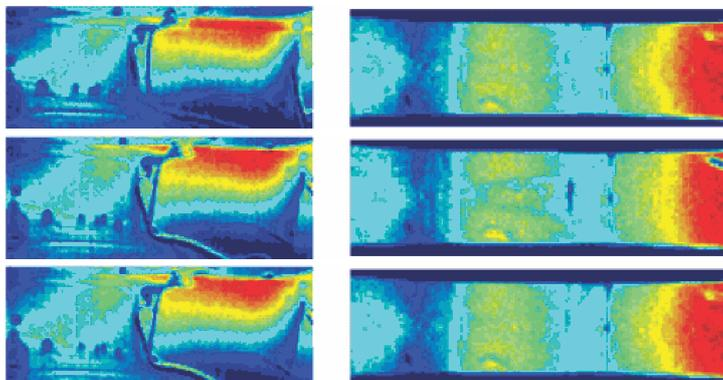
Figure 5: Left shows scans of the main landing gear pockets and right of the bonded metallic repair. Top, middle and bottom rows correspond to 0, 2599 and 5198 airframe hours respectively.
