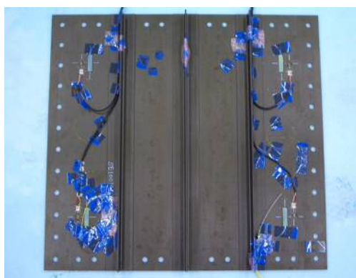
Figure 2: CFRP stiffened panel for simulated vibration test (Looking from stringer side)
