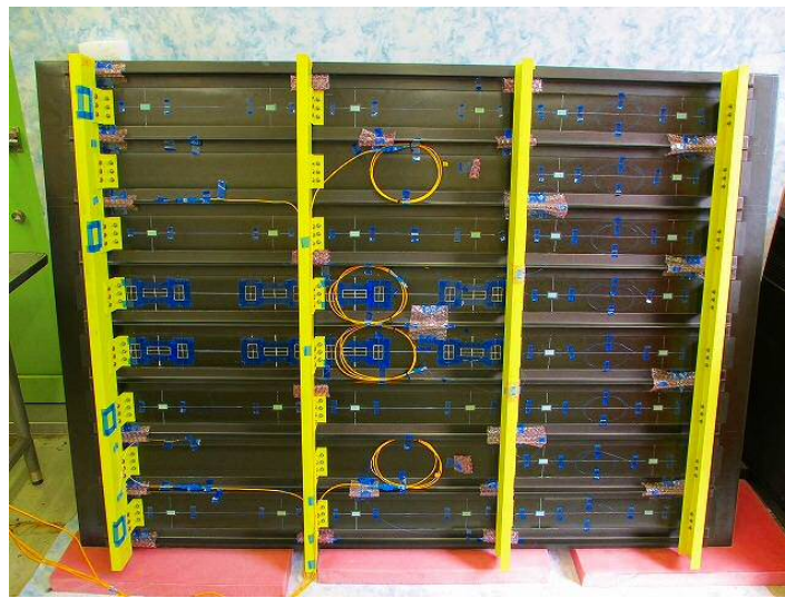
Figure 6: CFRP stiffened panel (Looking from stringer side)
