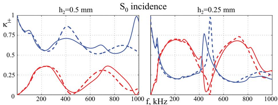
Figure 3 : Transmission (blue) and reflection (red) coefficients  $\kappa_S^+$  and  $\kappa_S^-$  obtained within LEM and beam models (solid and dashed lines, respectively) for the  $S_0$  mode in notched waveguides of web thicknesses  $h_2 = 0.5$  and  $0.25$  mm;  $h_1 = 1$  mm,  $\Delta x = 5$  mm.
