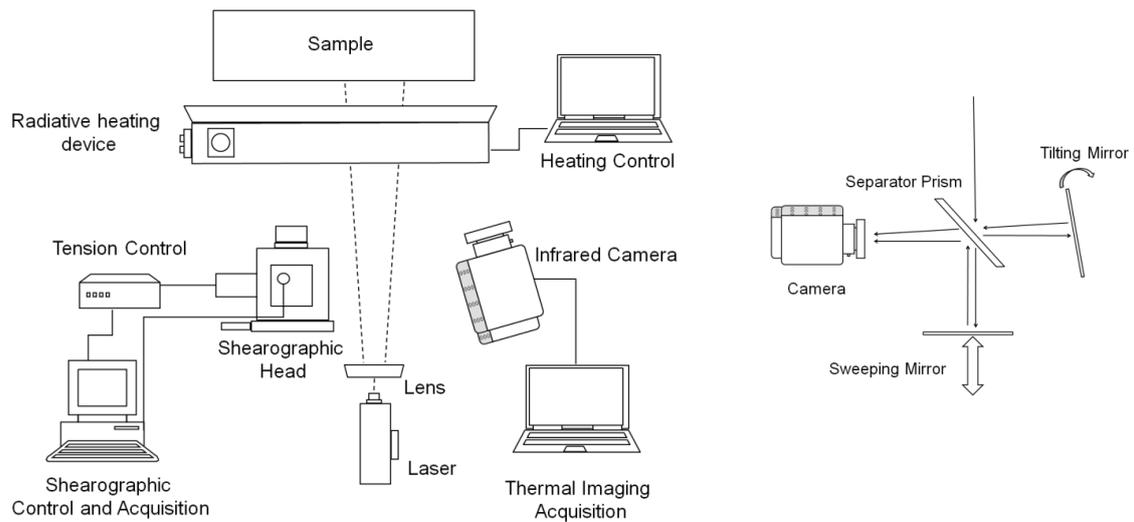
Figure 2: On the left, the schematic of the experimental setup of the simultaneous use of shearography and thermography. On the right, the detailed schematic of the shearographic head.
