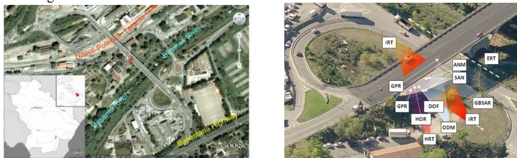
Figure 4: Location of Musmeci bridge in an aerial view (left) - Locations of sensors on the Musmeci Bridge in an upper view (right)
