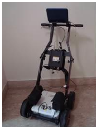
Figure 1: GPR system available at IREA-CNR equipped with the dual frequency antenna system working at the nominal central frequencies of 200 MHz and 600 MHz.
