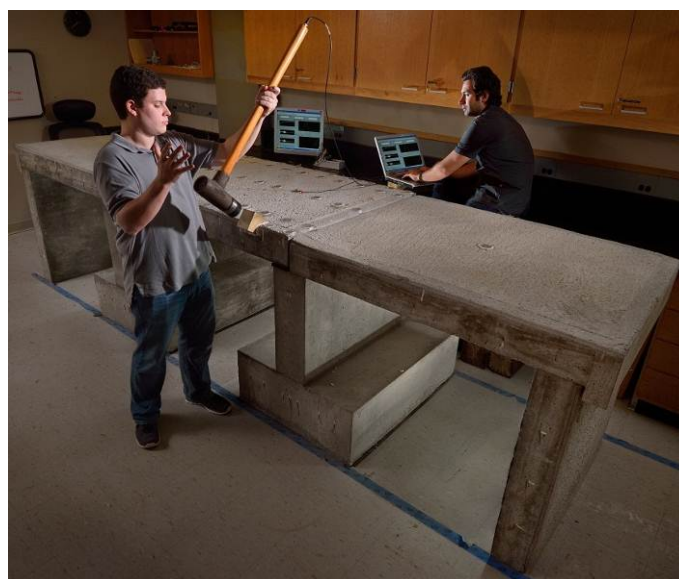
Figure 3: Graduate students performing impact hammer testing on the scale model bridge
