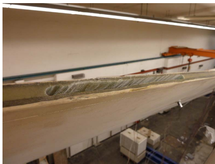
Figure 2: The artificial trailing edge damage introduced in the 34m blade
