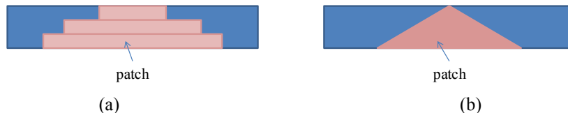
Figure 2: Bonded patch basic concepts: (a) Stepped lap joints. (b) Scarf lap joint
