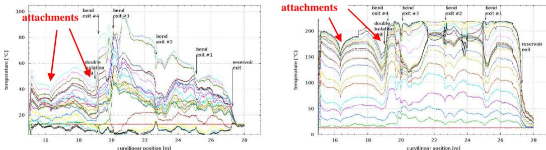
Figure 12: Distributed temperature measurements on first day (left) and second day (right)
