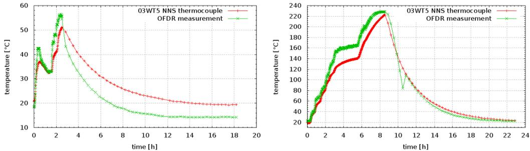
Figure 11: OFDR measurements compared with 03WT5 NNS thermocouple (left: 1<sup>st</sup> day, right: 2<sup>nd</sup> day)
