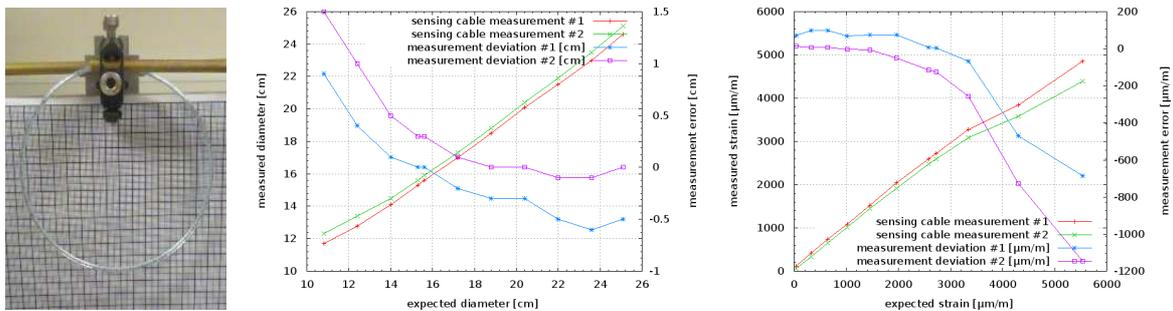
Figure 3: Curvature radius (centre) and strain measurements (right) with experimental set-up (left)
