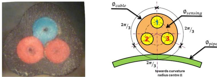
Figure 2: Strain sensing cable manufactured by Acome™, devoted to curvature radius & strain measurements
