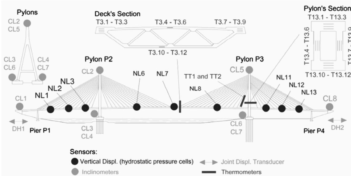
Figure 4: Monitoring system installed on Guadiana River bridge
