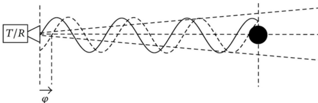
Figure 1: Working principle of interferometry
