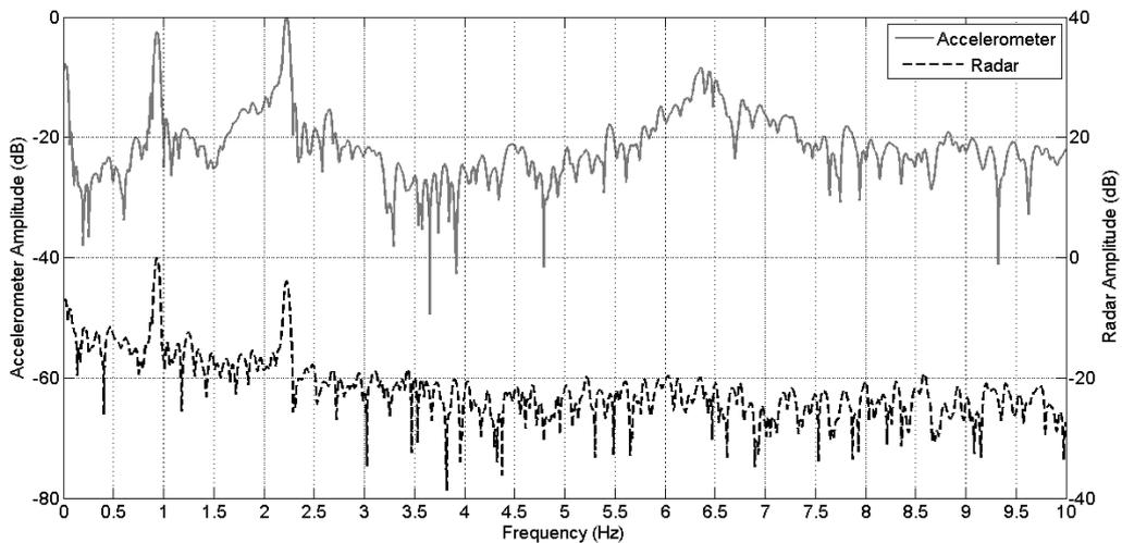
Figure 5: Street light analysis. Comparison between 40 s of accelerometric and radar data
