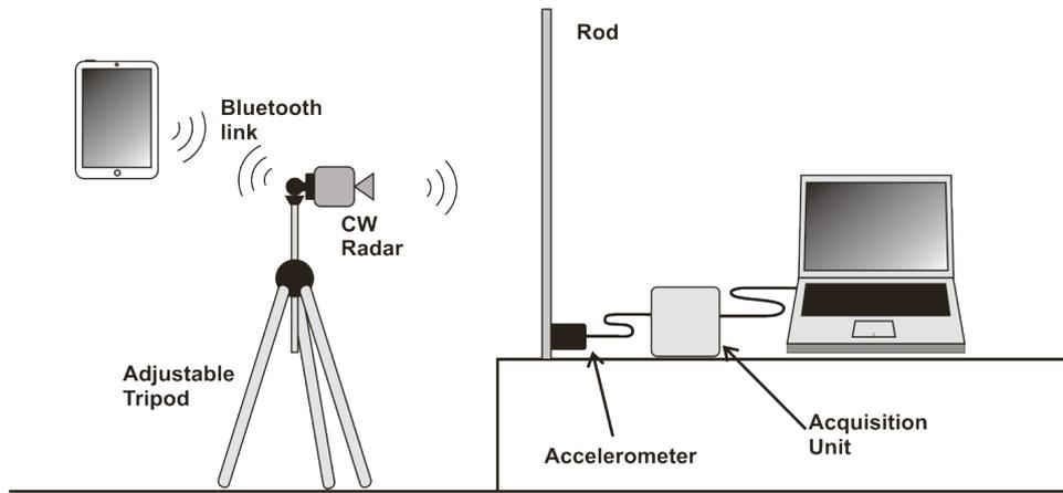
Figure 2: Experimental setup for rod oscillation measurement
