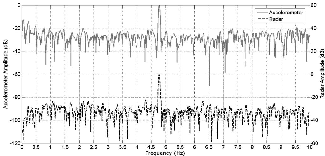
Figure 3: Rod analysis. Comparison between 40 s of accelerometric and radar data
