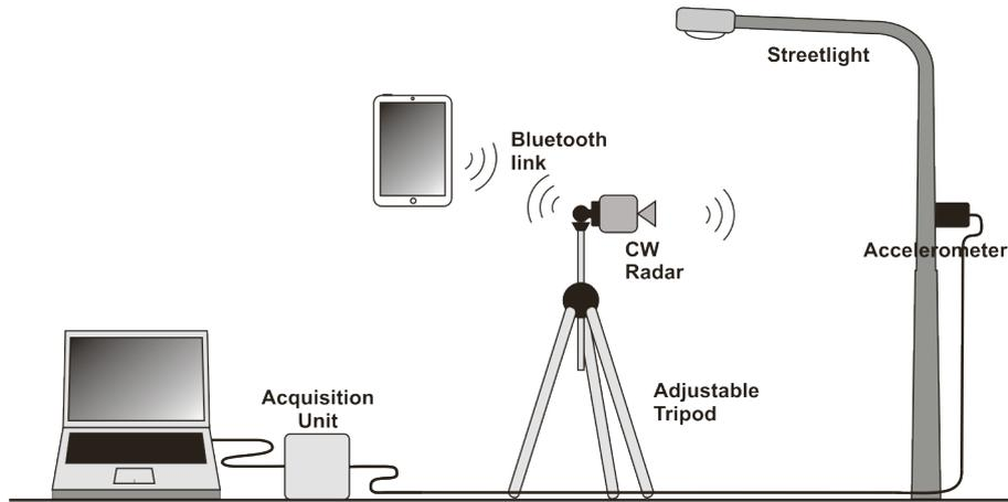
Figure 4: experimental setup for street light oscillation measurement
