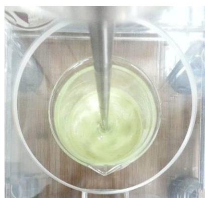
Figure 3: Piezo-paint in the vacuum desiccator.
