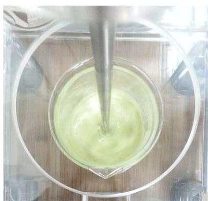
Figure 3: Piezo-paint in the vacuum desiccator.
