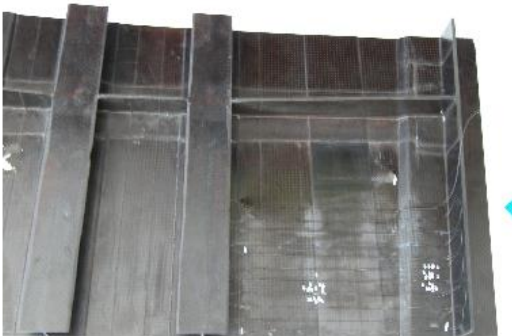
Figure 9 Cured CFRP structure, with bonded optical fibre
