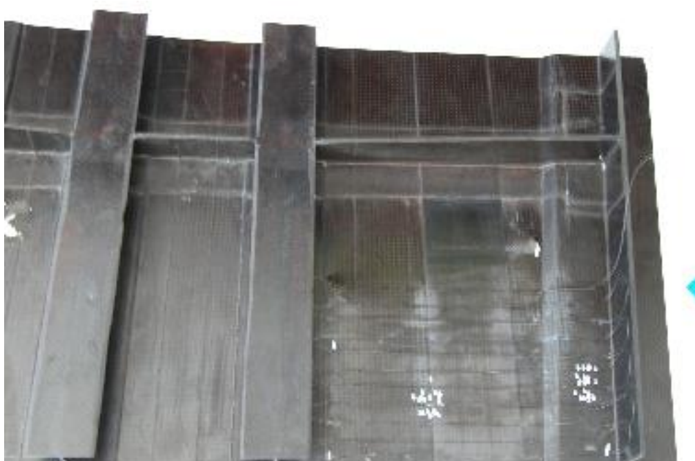
Figure 9 Cured CFRP structure, with bonded optical fibre
