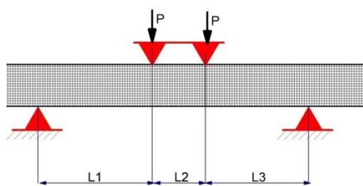
Figure 3. Four-point bending beam
