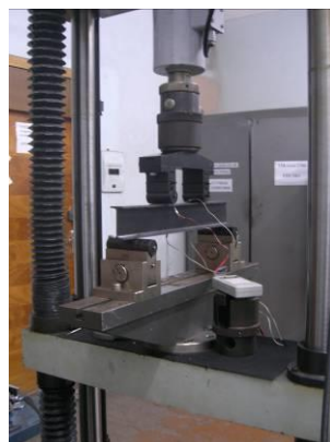
Figure 4. Four point bending experimental system
