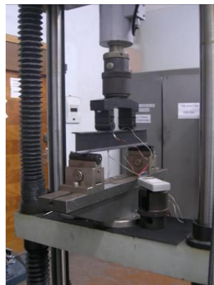
Figure 4. Four point bending experimental system
