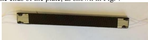
Figure 7. Composite plate with surface-mounted transducers.
