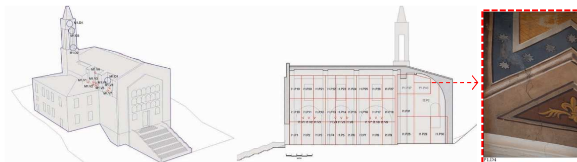
Figure 1 : 3D model and photographic mapping of the Church in Giglio Porto.
