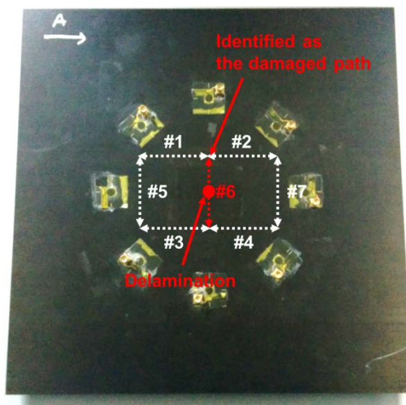
Figure 7: Damage identification results on the composite plate. As it has been shown in Figure 6 (b), only the path passing through the delamination (#6) is identified as the damaged path.
