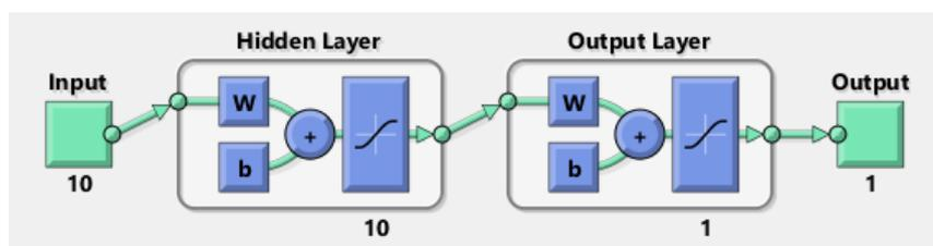
Figure 4 : Neural network created for damage detection purposes.
