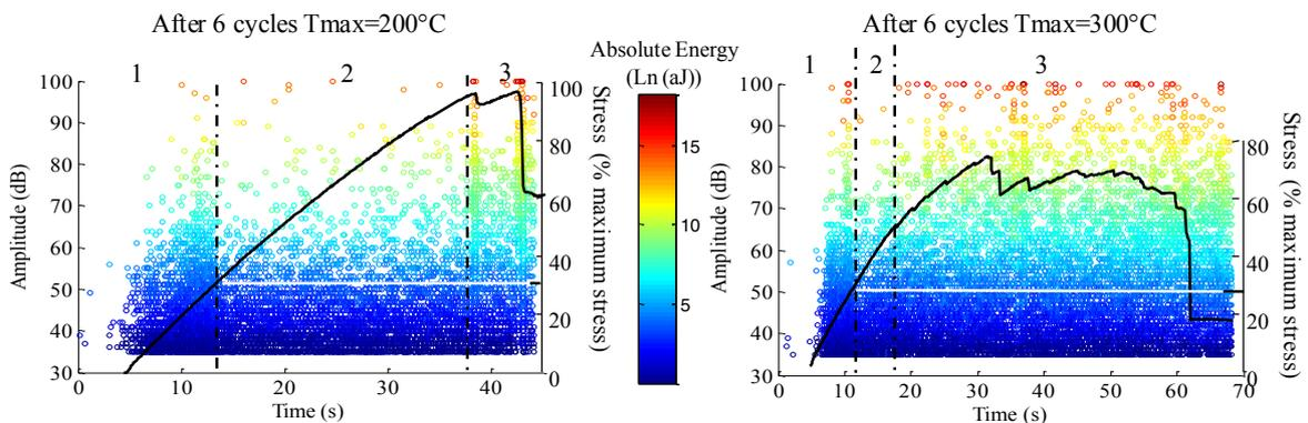
Figure 9 : Amplitude and energy of the AE signals with the stress curve of the 200°C and 300°C cycled specimens respectively.
