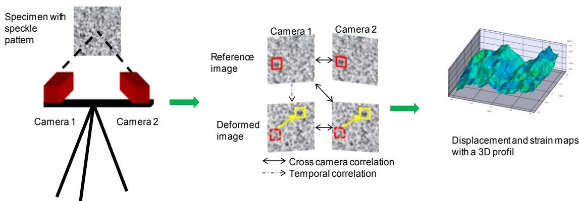
Figure 2 : Schematic view of the process of DIC
