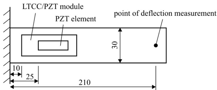
Figure 5: Sketch of beam set-up; the LTCC/PZT module and the PZT element are positioned on top of the metal sheet centred to its symmetry axis.
