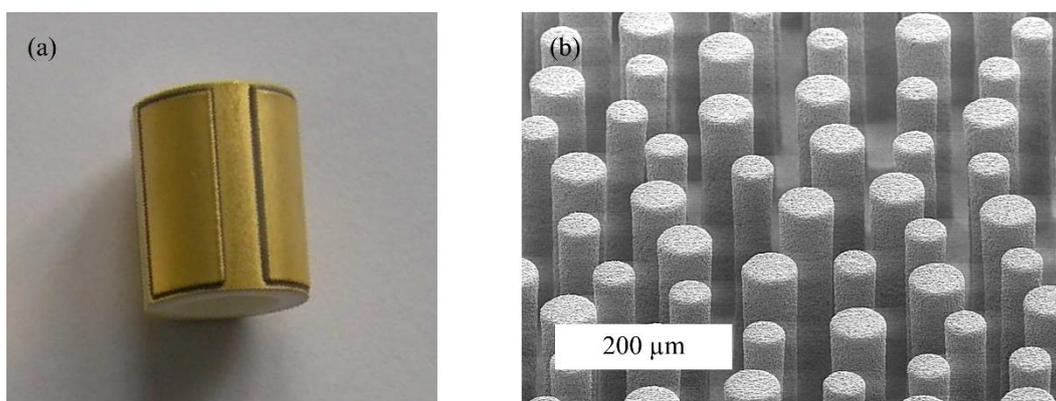
Figure 1: (a) PZT thick film with electrode layers on  $\text{Al}_2\text{O}_3$  cylinder [11]; (b) fine scaled PZT rod structure for piezoelectric 1-3 composite manufactured with the soft mold process [12].
